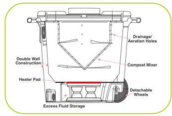
The option to purchase a model with a Heater pad in the bottom of the chamber for improved composting conditions during cold winter months.
