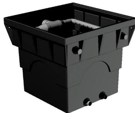
The filtration tank should be at least partially dug (at least 500mm deep) into the ground. The tank should be laid on a bed of sand with a 1-2% incline towards the outlet pipes.
