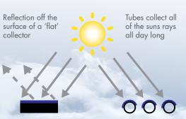
Evacuated tubes catch & keep the sun's radiation, & reflect less of the sun's energy.
