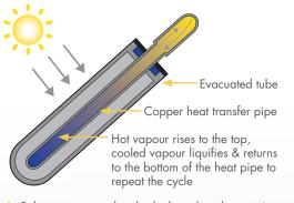
▲ Solar energy absorbed by the heat pipe inside the tube.
