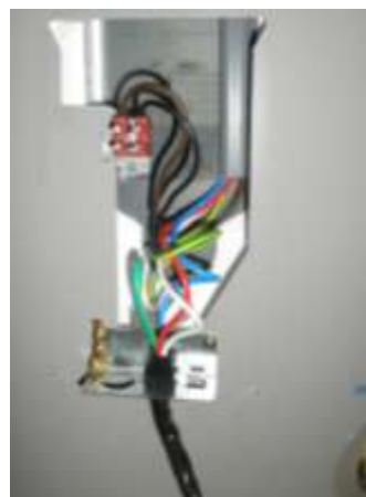
Step 3 withdraw the power cable
